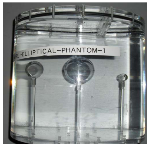
Fig. 5. Elliptical phantom used in physical phantom experiments showing three spheres of different sizes.
