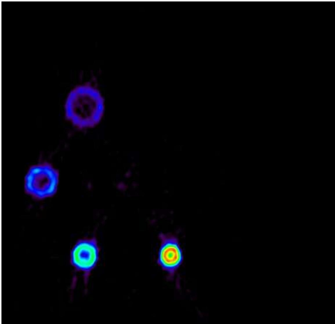
Central slice of image quality phantom reconstructed with STIR for the Discovery ST scanner geometry showing heavy attenuation in the center of the spheres.
